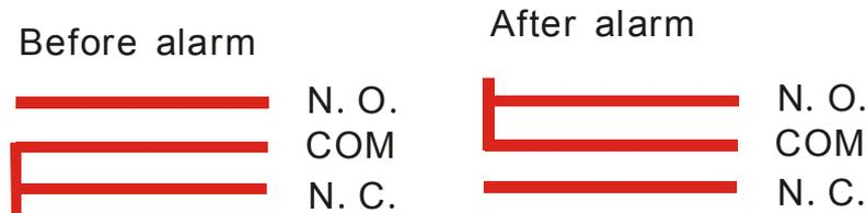
Fig 2.9 Relay Output Status
