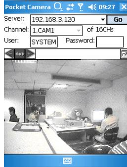
**STEP7** Camera1 is the default display after login. Change the camera in rolling-down menu of “Channel”.
