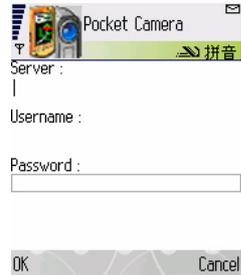
**STEP8** Input the server's address, ID and password respectively. And click OK to login the DVR.
